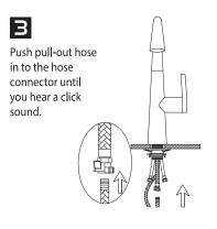
Proper installation of the hose weight kit will ensure that the spray head retracts smoothly. On the spray side of the hose, measure 15" down from the body of the faucet. Install the hose weight kit at this point. Pull out on the spray head. It should move easily and retract smoothly. Reposition the hose weight kit as necessary.
