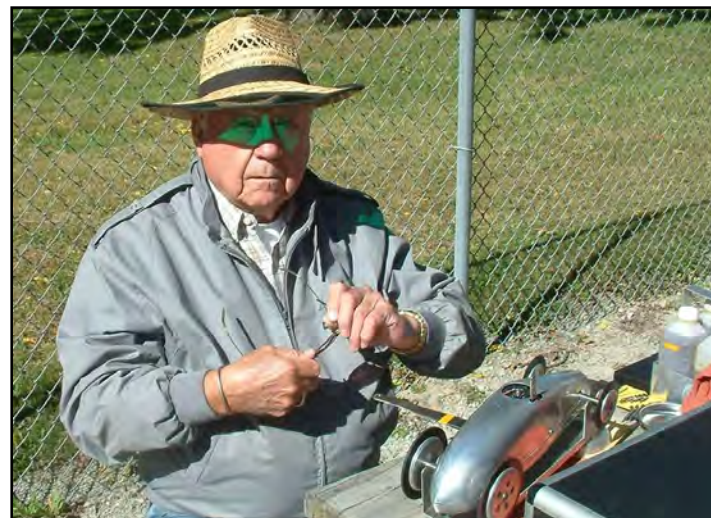
Don Ulrich readies his hand-formed aluminum, Rossi 45-powered HB1 car.
