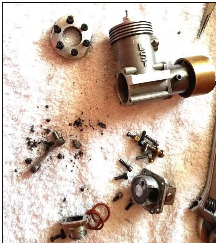
On June 24, at Whittier Narrows, John Newton was running his Russian car with a 2.5cc Stellings engine from Lithuania. He had installed a new Profi BE/CU piston and sleeve. It got up to 130 mph when the new piston disintegrated as shown in the photos.
