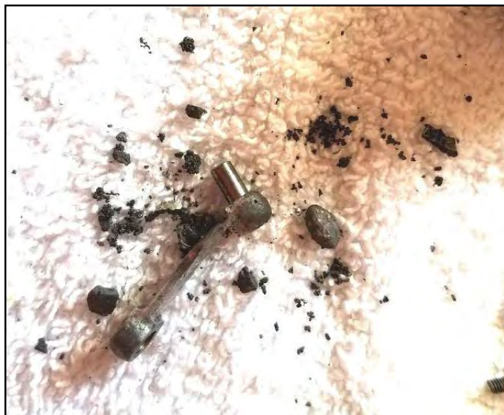
On June 24, at Whittier Narrows, John Newton was running his Russian car with a 2.5cc Stellings engine from Lithuania. He had installed a new Profi BE/CU piston and sleeve. It got up to 130 mph when the new piston disintegrated as shown in the photos.
