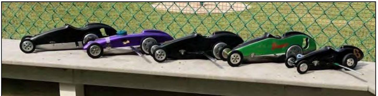
(Below) A lineup of cars John Ellis built that were run at the Memorial. Three Kuebler/Ellis Eagle-powered Class 3A cars, a Kuebler/Ellis Ellis-powered Class 10B (second from left), and a Kuebler/Ellis Dooling .29 powered Class 7B car. He was a prolific builder of quality cars and engines.
