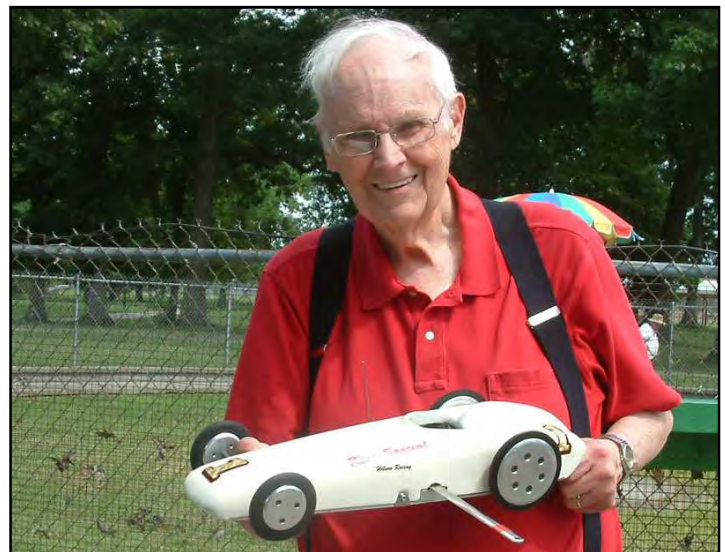
Walt Wilson with his electric-powered "Kiss Special". It managed to turn 129 riding on ground-down tires, hubs, and tail skid. It needed throttle programming adjustments.
