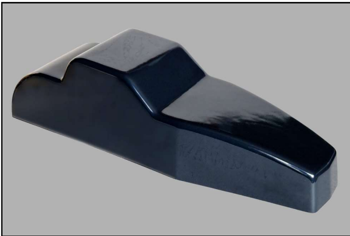
One of the fiberglass bodies for the new electric entry-level car the Phillips brothers are developing.
