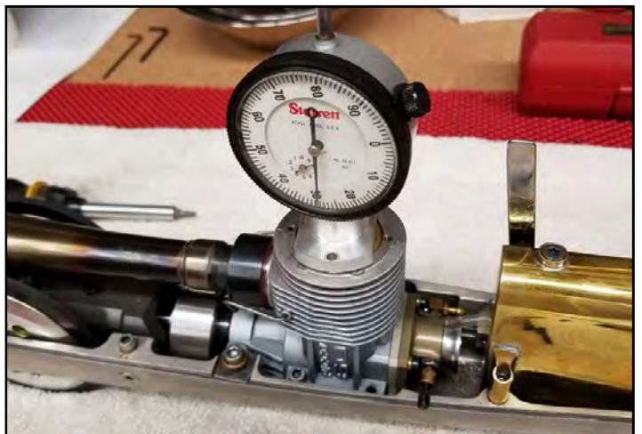
Dave Lundegard checks deck clearance on the Picco in his 10cc Duran car.
