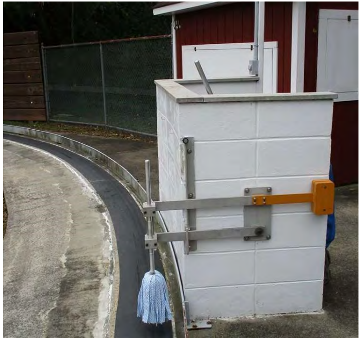
Thanks to Bill Siry, a string mop replaces the bristle broom at the New York track.
