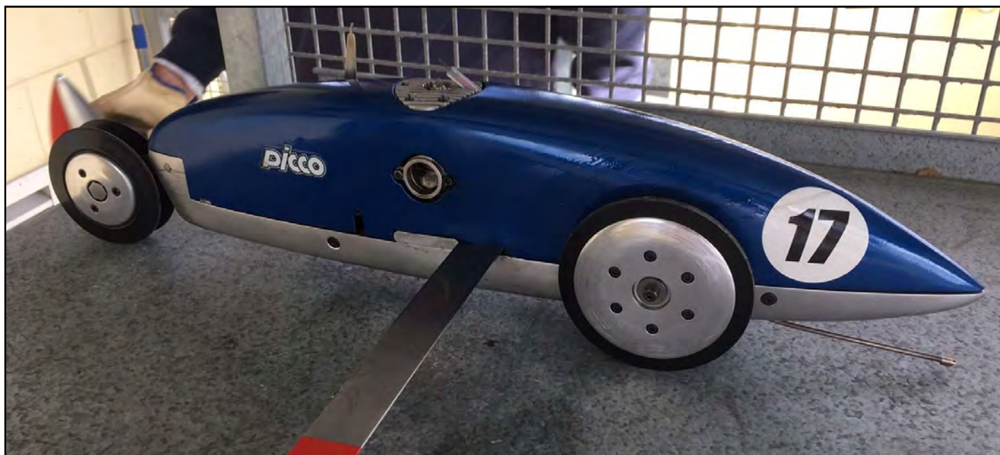
Scott Clydesdale's very fast 10cc C Grade Chadwick car powered by a Picco P-60 turned 162.757 MPH, and that's on 80/20 WMCR fuel .
