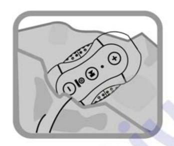
5. Use cotton buds to thoroughly wipe off all remaining water droplets from the joint between the front and rear clip.
