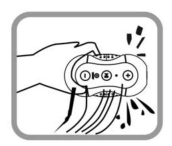
4. Use a clean cloth to wipe off any excess water. Be sure to use a cloth that is free of salt residue and doesn't have any loose fibers.
