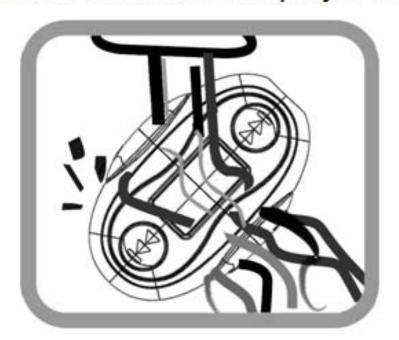
2. Immerse the player for around 2 or 3 minutes in pure water to remove any salt or dirt.
