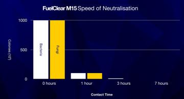
The time to achieve eradication varies according of the extent of the contamination and the type of microorganism present. Typically, as the graph indicates, within 24 hours of treatment the fuel will again be fit for use.
