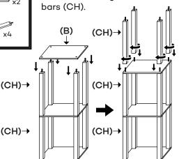
STEP 4b Screw-in the upper long bars (CH) through the double-sided screws of the lower long bars (CH).
