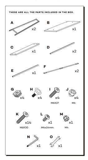
STEP 1 Insert the square tube insert<sup>(G)</sup> to the bottom of the desk legs.
