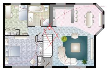
using a compass, draw circles on the drawing by placing the centers of these circles in the corners which are furthest from the center of your home. For example, for a 30 ft (9.1 m) hose, use radii of 3.3 in (8.5c m);
