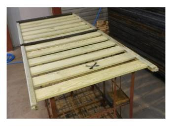
**Step 4**Remove the existing staples on the frame back side.
