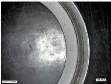
Figure 19. TE bearing outer race (post-drop test), with a mixture of fresh grease and dark particles
