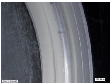
Figure 20. TE bearing outer race after cleaning shows minimal wear
