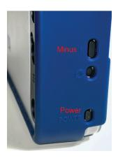
o If the LED is not dark blue, hold the Minus Button '-' on the side of the device for 30 seconds. Wait for one minute. If the light does not turn dark blue, please contact VetGuardian Support.
