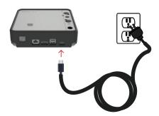
b Hold the Power Button on the side of the device for 3 seconds. After a minute, a corner LED light will turn dark blue indicating the device is in setup mode.
