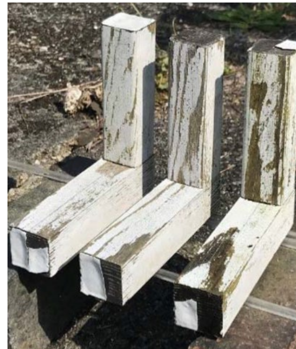
The acetylated L-joints after 20 years of exposure
