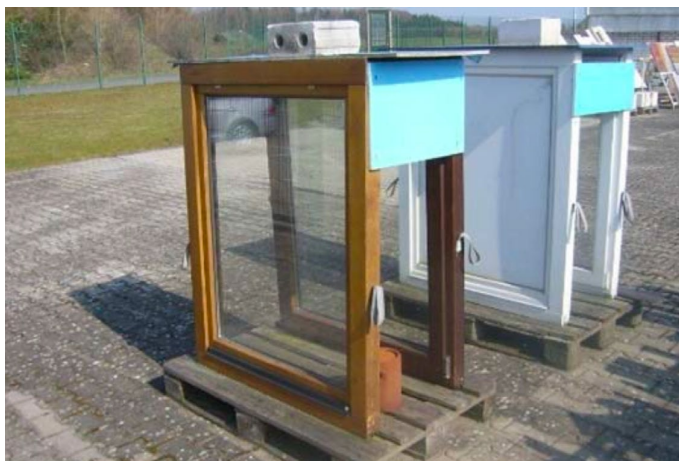
The test rigs after 10 years of exposure
