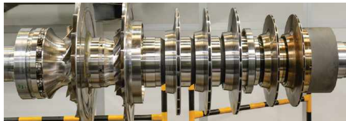
HPRC is a high-speed rotor-compressor with small footprint and high-performance stages for various applications including hydrogen
