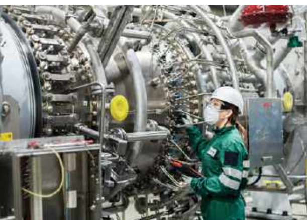
NovoLT™16 gas turbines can burn up to 30% vol H 2 in DLN mode, with design enhancements moving toward 100% H 2
