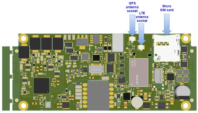
External antennas can be connected directly to u.Fl connector or via u.Fl to SMA adapter. While connecting antennas, users should follow antenna connection rules described in a datasheet provided by antenna manufacture in order not to lower device RF performance.
