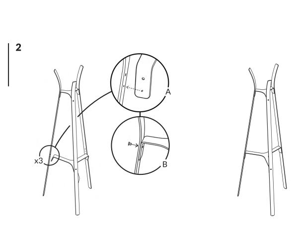
A - Fit the bump into its hole first.
