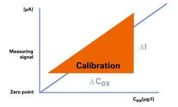
The calibration is based on Faraday's law and a flow measurement.
