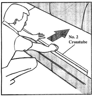
If sleeper unit does not come off the J-slot screws during closing, grasp No. 2 Crosstube shown in illustration and push toward back of sofa. (You may need to go to each end and lift unit off.)
