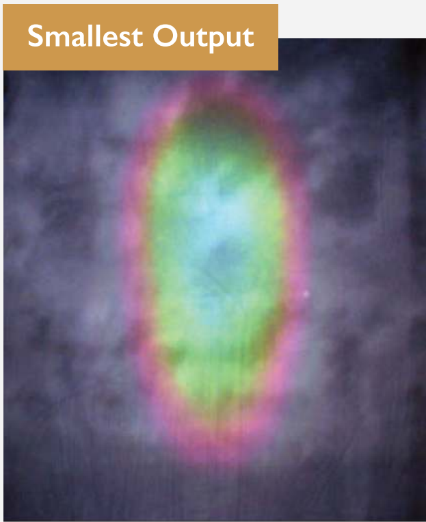
Carbon Panel Emitter 'Panel Type' Carbon-based heater displayed the least infrared output.
