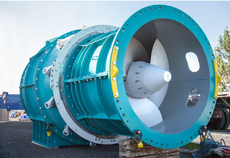
Above left: D190 RHT prior to installation. Above right: a variable-speed RHT design with adjustable wicket gates can match Kaplan turbine efficiency between about 65-100% of full load. RHT efficiency can exceed conventional propeller turbine efficiency across a wide range of load.
