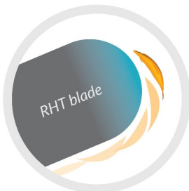
Thick, Curved blade (deflects fish around)
