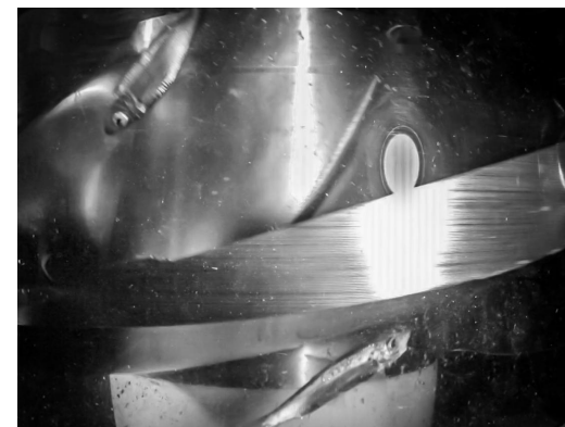
Below left: The blade shape that characterizes FishSafe™ RHT designs both reduces the likelihood that runner blades will strike fish and also reduces the severity of strikes that do occur. Below right: A still frame from high-speed video shows the safe passage of juvenile alosines through a D55 RHT.
