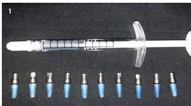
Fig 1. Subgroup 1B (n=10) – Titanium abutment / Titanium implant – Sealant applied at IAI.
