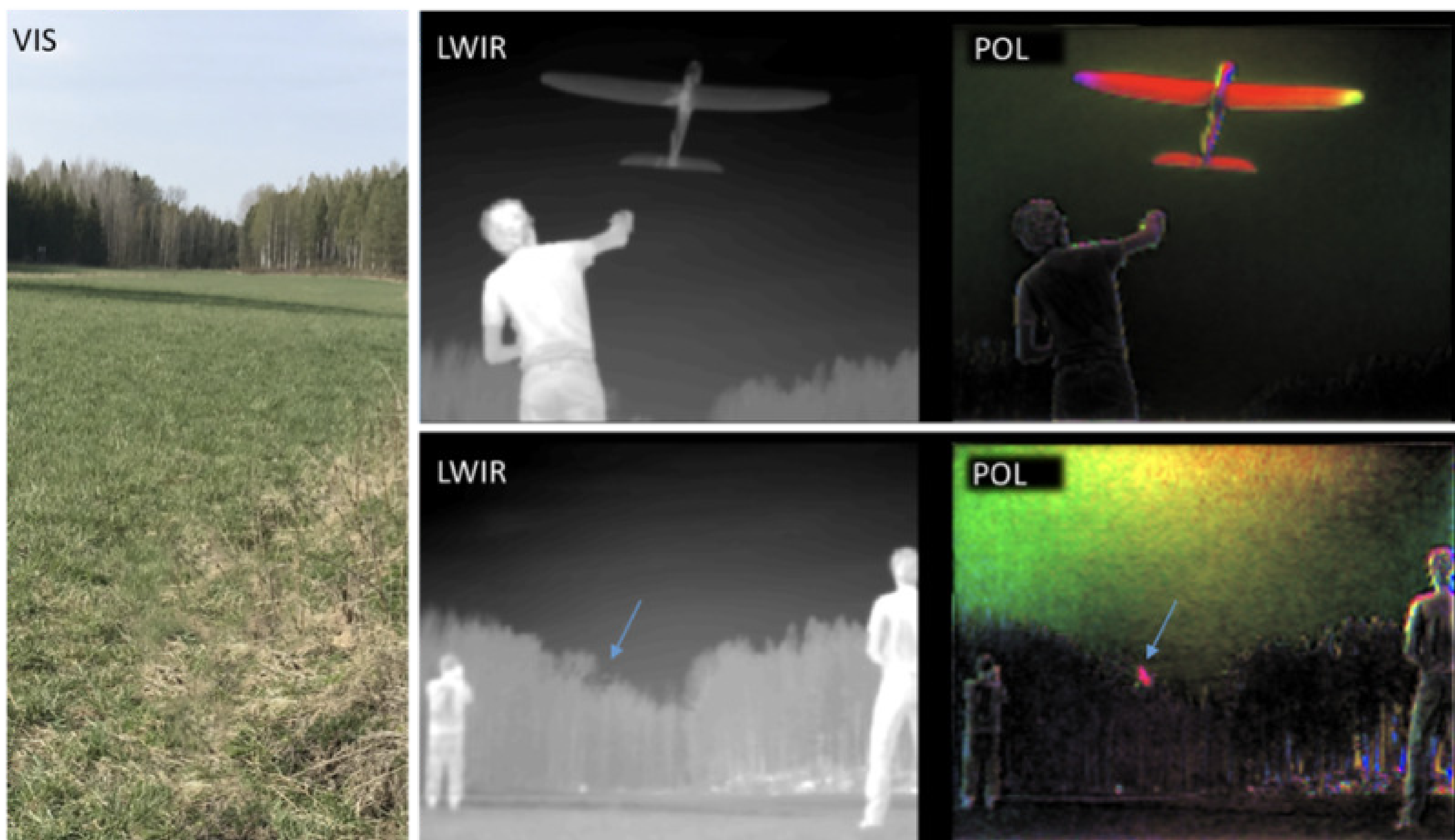
Long range / small UAV increased detection
