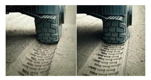
Although most often used in conjunction with all-wheel drive, CTIS has proven so effective that non-all-wheel drive vehicles equipped with CTIS can actually outperform all-wheel drive vehicles without CTIS in many soft-soil conditions. As a result, nearly every tactical military vehicle worldwide is equipped with CTIS.
