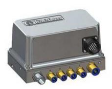
**Electronic Control Unit (ECU)** is the "brains" behind the CTIS system, processing driver selections, provides decision making and logic execution. The ECU communicates with the vehicle CAN Bus, monitoring power, speed, etc., sends commands to the PCU which directly controls the wheel valves and senses tire pressures from the PCU. Electronic circuitry is completely sealed resulting in a rugged, environmentally robust package.
