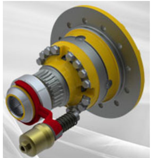
Figure 1: Differential case half showing shift collar, shift fork (red), and actuator.
