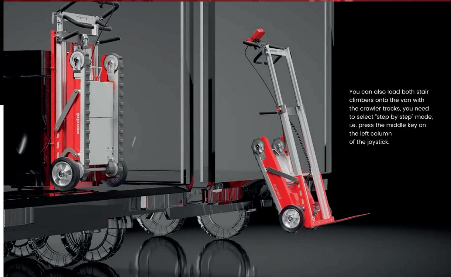
You can also load both stair climbers onto the van with the crawler tracks, you need to select "step by step" mode, i.e. press the middle key on the left column of the joystick.
