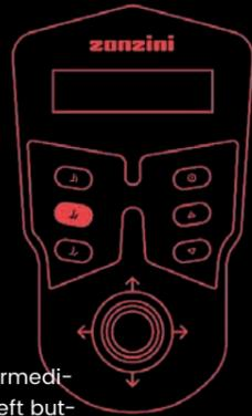
Crawler tracks in intermediate position. Middle left button of the joystick. It is possible to go up and down the step using the pair of teeth of the crawler tracks gripping the step. This is the "step by step" mode that the operator uses to keep the load balanced.
