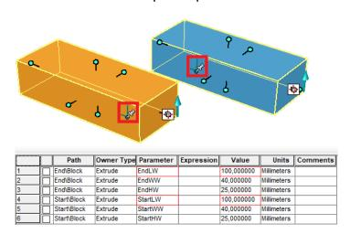
When the blue model *Length* dimension (*StartLW*)) changes from 50 to 100 in the Parameter table, it will update the model in the Anchor Point *Start* direction – it becomes longer on the right side (or the negative X direction).
