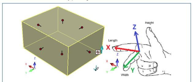
The <u>long leg</u> corresponds to the <u>positive Z</u> direction, or the <u>right-hand thumb</u> if you will. The <u>short leg</u> corresponds to the <u>positive X</u> direction, or the <u>right-hand index</u> <u>finger</u>. The <u>positive Y</u> direction lacks a "visual leg shape" but you can visualize it as the <u>middle finger of the right hand</u>.
