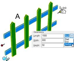
The fence can only by modified in one direction -> the opposite side of the Anchor Point.
