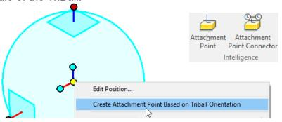
The main difference between the two is that the Attachment Point created by the TriBall isn't automatically associated with the object it is attached to, which it will be when created with the AP tool or dropped from a catalog. Since a face or point will light up in green on drop, there will also be an associativity created to that face or point.
