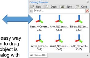
Attachment Points can also be reused in an easy way through catalogs. Use the <u>right mouse button</u> to drag an AP into a catalog. Make sure the correct object is selected before dropping an AP from the catalog with the left mouse button.
