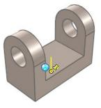
When the TriBall is activated, it is now the Anchor Point that is moved and reoriented. For example, if you want the origin point of a part in a certain corner, instead of the center of the part where it often starts off.
