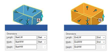
The *Length* parameter named \*\*\*LW (short for \*\*\*Length Write) is connected to the Sizebox *Length* handle in the IntelliShape Properties.
