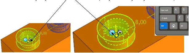
For *Patterns* created by the TriBall, you must also activate a certain setting under the Options, or else the dimension will be tied to the object (Feature, Part or Assembly) instead of the Anchor Point of the Pattern.
