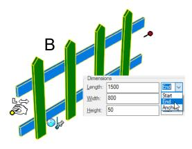
It is no longer the position of the Anchor Point that controls the change of the L handles, but the orientation (of the visual legs) alone. The Anchor Point will also change its position and follow in the direction of change and keep its relative position within the Sizebox of the Assembly.
