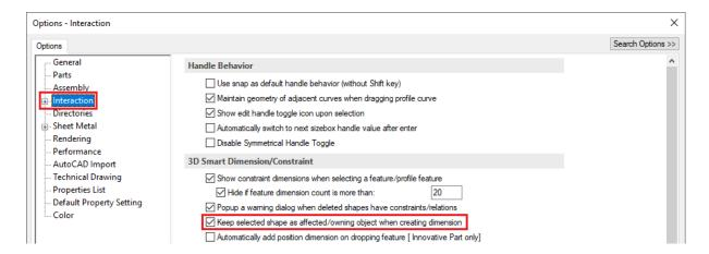
The setting can be found under *Interaction* and is called *Keep selected shape as affected/owning object when creating dimension*. Without this setting active it is not possible to tie dimensions to the Anchor Point of Patterns.
