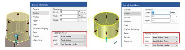
In the case of a symmetrical shape with the Anchor Point outside the center (right image above) it could use **About Sizebox Center** only on the **Length** and **Width** handles. It will ignore the position of the Anchor Point and only use the Sizebox handles relative to each other.
