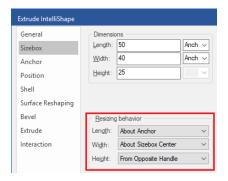
Under the *Intellishape Properties* you can manage the <u>three basic rules</u> on how the Sizebox L-, W- and Z-handles should behave when dragged and the Anchor Point is involved here as well.
