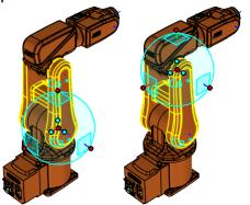
Using the [TAB] key, the TriBall can easily move between the AP's available on the selected object.
