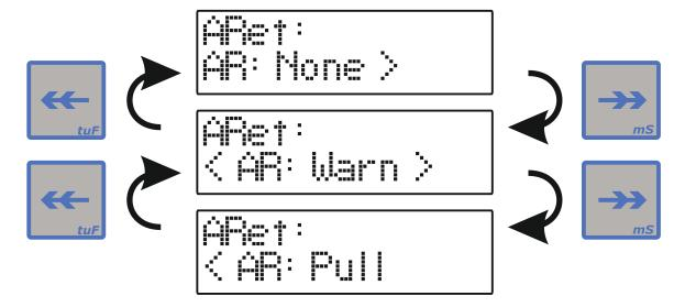
When the correct setting is selected, press the Enter key to store the data. The retention bar main menu item is now displayed.
