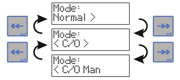
When the correct setting is selected, press the Enter key to store the data. The auto divert setting is now displayed.
