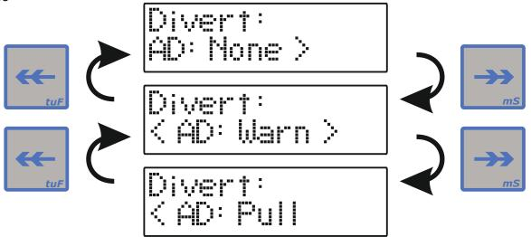
When the correct setting is selected, press the Enter key to store the data. The dump line invert setting is now displayed.
