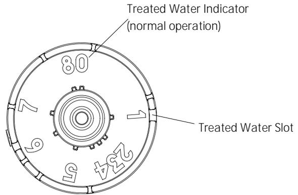
The corresponding slot for the number is positioned at the optical sensor which is approximately 90 degrees out of phase.
