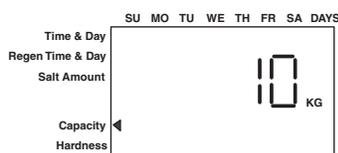
To have your system regenerate on demand, set your system's capacity (P7) to the appropriate factor. On the 762, it will read Kg, but you will actually be working in ppm of iron.
