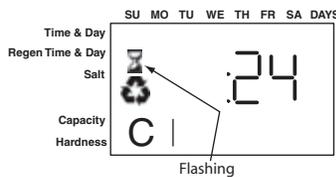
The controller will indicate that the motor is turning the camshaft to the cycle C1 (Backwash) position by flashing an hourglass. The controller will display the total regen time remaining.
