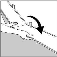
3. At the end of the first row: Leave a gap of 10 mm to the wall to avoid any damage while installing your floor and measure the length of the last plank to fit. Insert the short side and tap it closed, using a pull bar.
