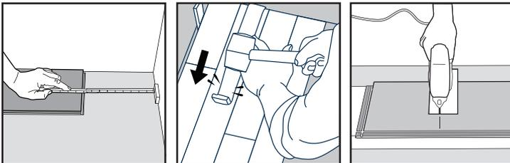
4. Starting second row: Rows can be started with end cuts if the cut plank is at least 30 cm long. If end cut is used for subsequent row a stair step pattern is established. Starting planks of random lengths will create a more aesthetic random stagger. Short end joints must not be closer than 20 cm to each other.
