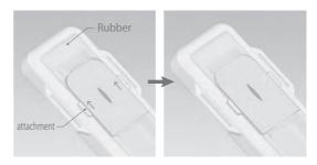
②Holding the lugs, slide the skin unit to the opposite direction so that its shorter tenon is inserted in the section of the smaller rubber.
