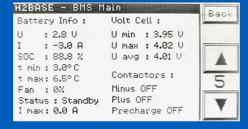
Submenu for the buffer battery
