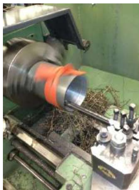
Figure 20. Use of a lather to bore out a steel pipe for cylinders
