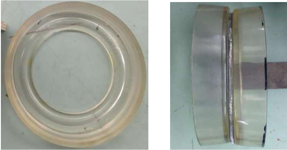
Figure 38. Injection molded seals
