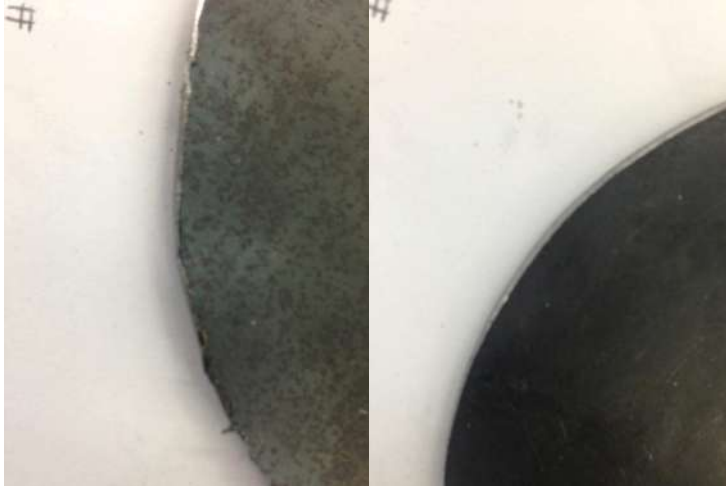
Figure 32. Left side is rough before filing. Right side is smooth after filing.
