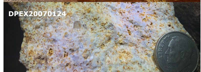
Diaspore is present in vuggy silica ribs on southwest flank of lithocap west of and structurally below quartz-alunite blanket
