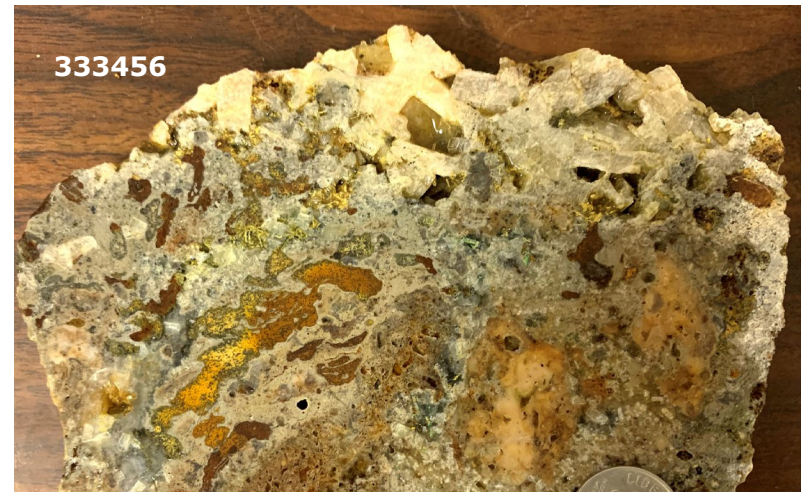
Vuggy silica breccia with barite infill cutting illite altered tuff. 0.27 ppm Au, 277 ppm Ag, 4080 ppm As, 6050 ppm Bi, 752 ppm Cu, 1320 ppm Sb, 430 ppm Sn
