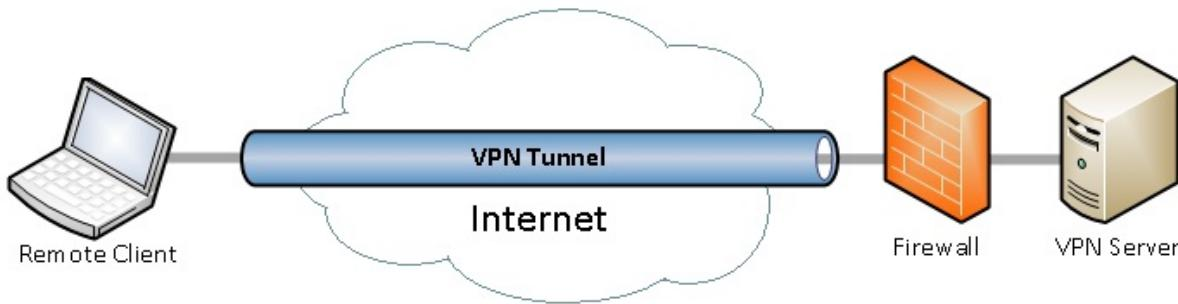
Because the VPN tunnel is a secured connection the internet connection on the remote client computer is terminated to force all internet traffic to go through the VPN tunnel.
