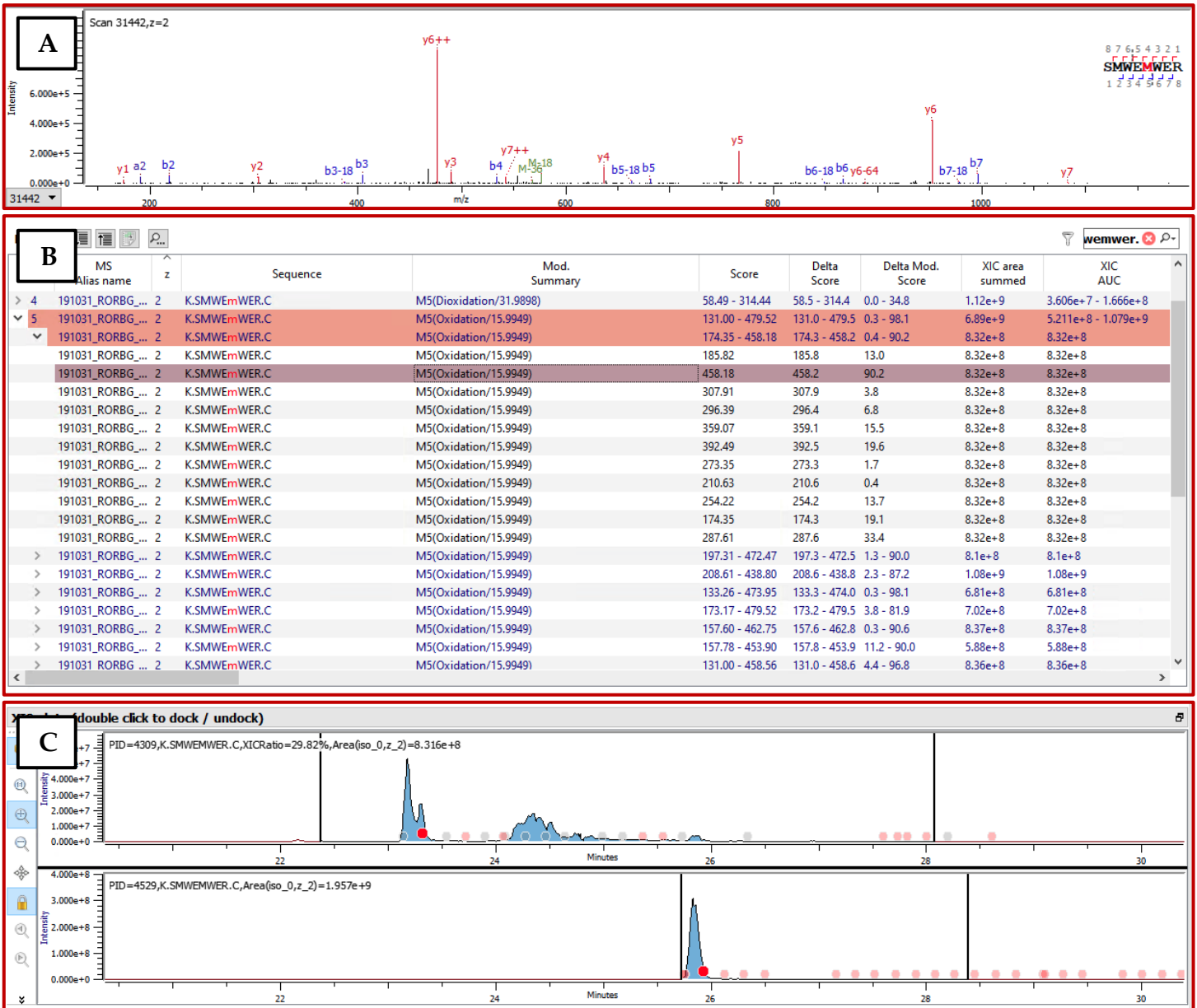
Figure 3: Protein Metrics Byologic will automatically generate a list of modified peptides which it identifies during a search. Localizing a specific modification to a particular residue is done by analyzing the MS 2 data ( Figure 3A ). A list of MS 2 hits that were identified as a modified residue will be generated ( Figure 3B ). Each hit will be assigned a “Delta Mod Score” which is a measure of the confidence in the assigned localization of the modification to a particular residue (shown as a red letter). Selecting a MS 2 hit shows where on the extracted ion chromatogram (XIC) plot the MS 2 data was collected. Figure 3C shows two XIC plots: the top corresponds to the modified peptide with the dark red dot showing the location of the selected MS 2 hit, and the bottom corresponds to the wild type, or unmodified, peptide. Selecting the MS 2 hits with the highest Delta Mod Score will allow the user to locate a particular peak on the XIC plot which corresponds to a localized modification.
