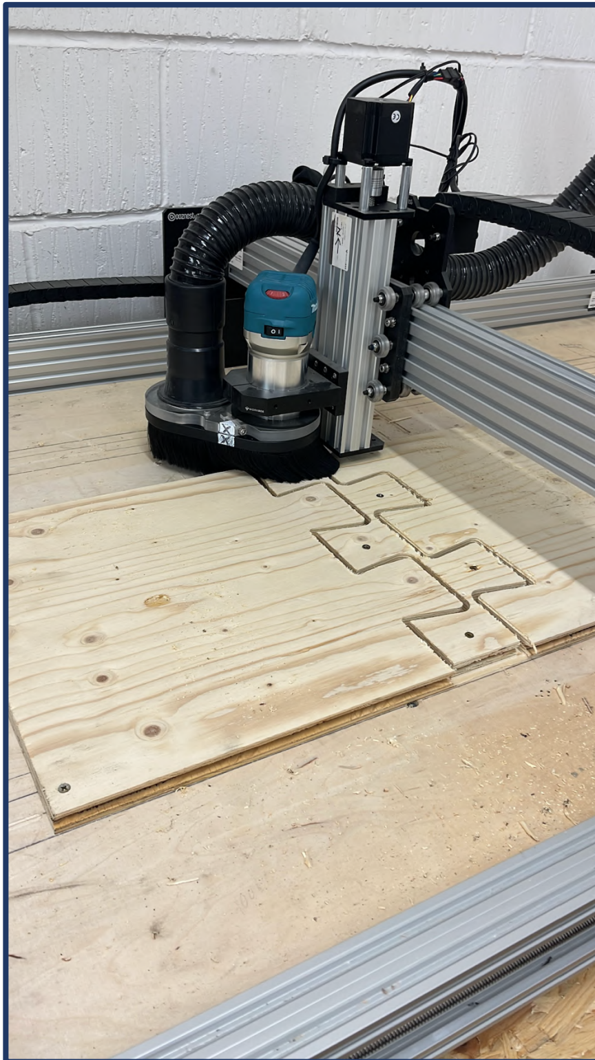
Figure 16: CNC fabrication of jigsaw joints
