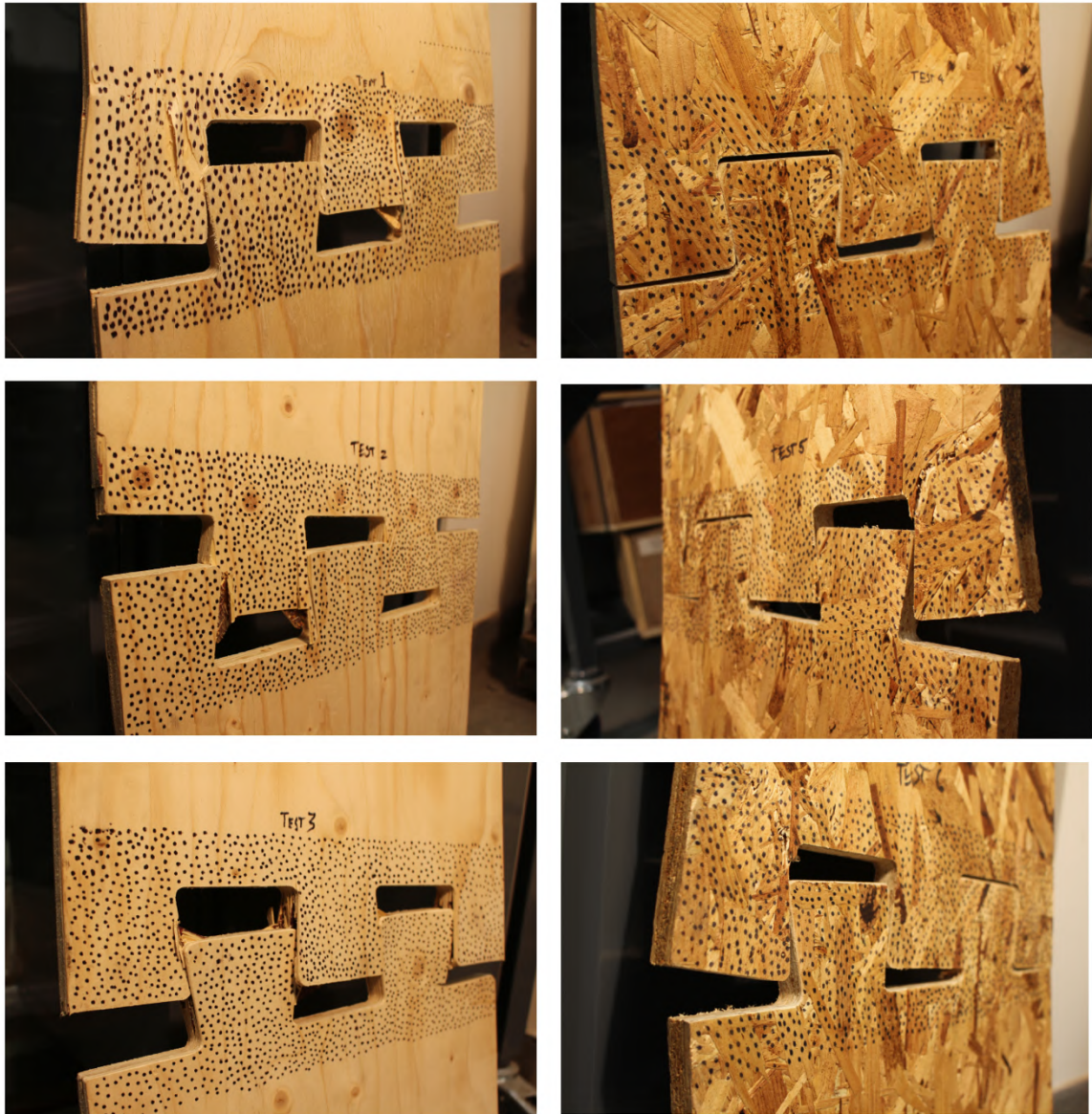
Figure 17: Jigsaw joint samples after failure (Left column: Plywood, Right Column: OSB)
