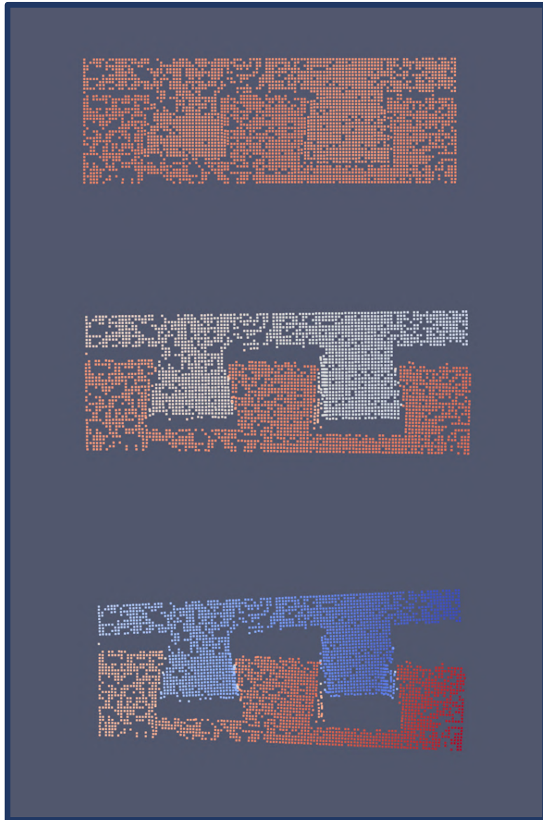
Figure 22: DIC visual showing plywood jigsaw joint deformation
