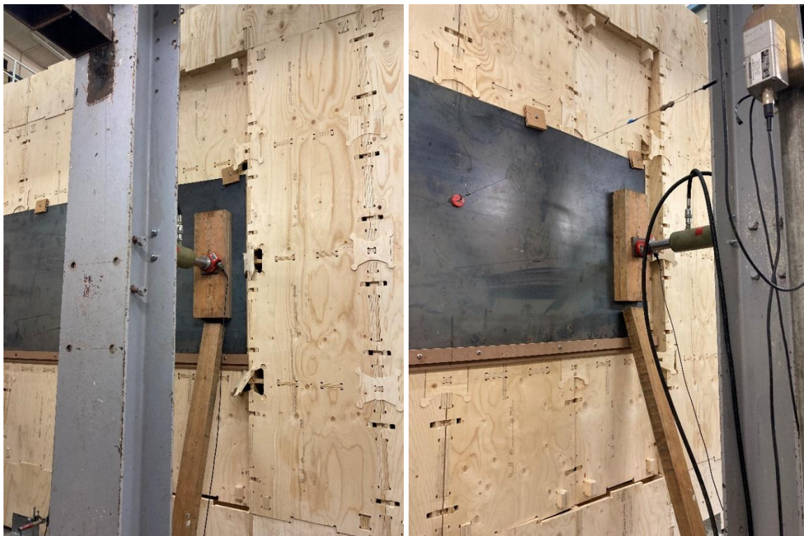
Figure 29 - Damage to the East Wall at Failure Loading
