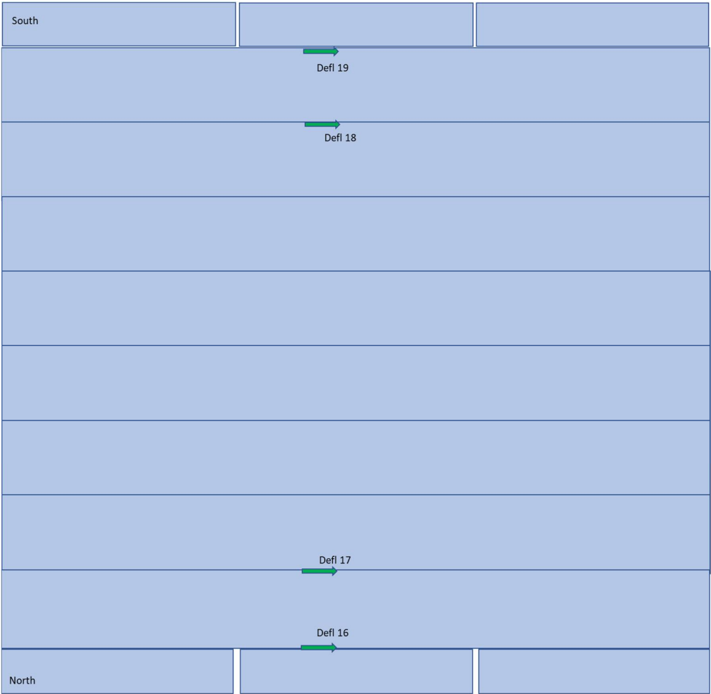
Figure 27 - Displacement Transducer Locations for Roof of the 3D Module Test
