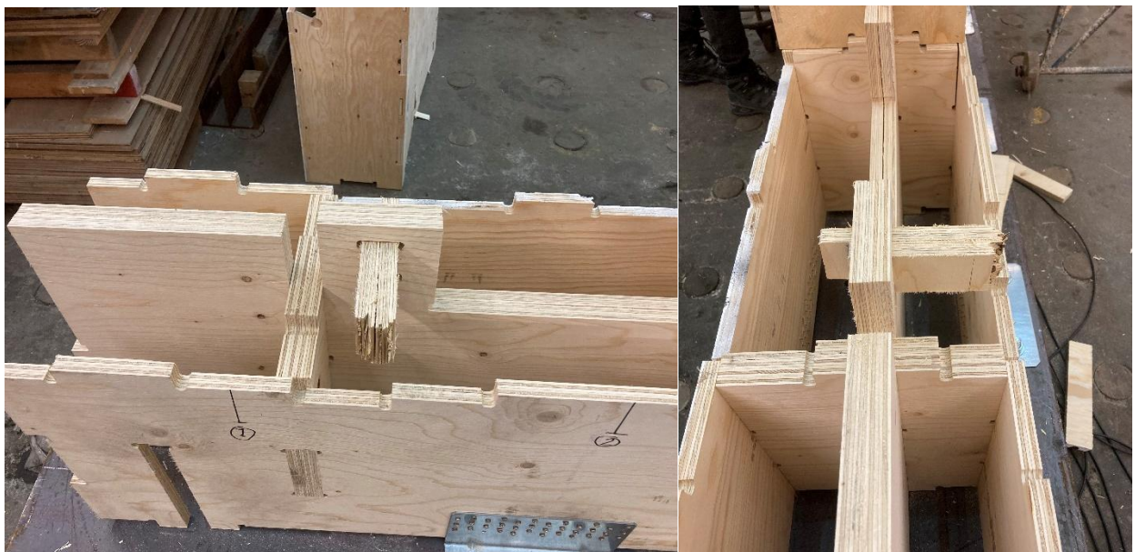
Figure 12 - Broken Pin at the Through wall peg
