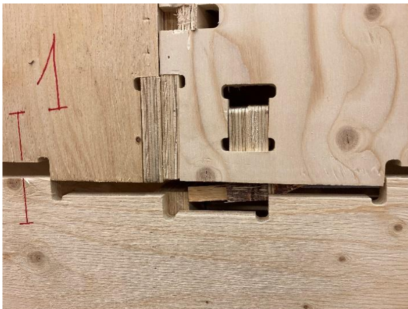
Figure 20 - Movement in Through wall peg
