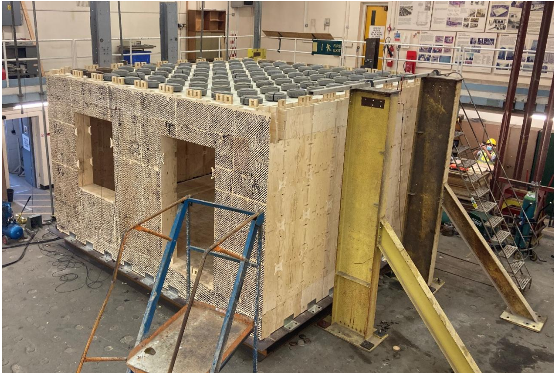
Figure 6 - 3D Module showing Roof Loading and Buffer Structure
