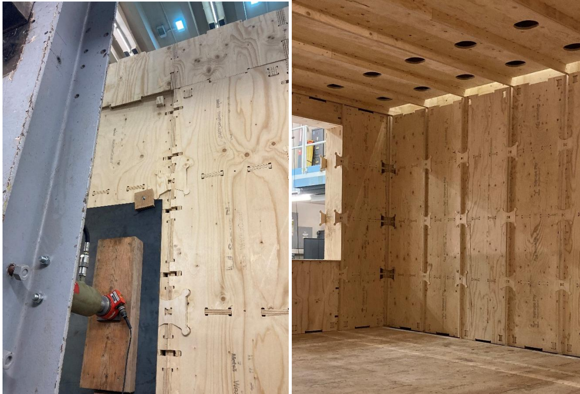
Figure 28 - Damage to the East Wall at 0.4F Loading showing Broken Bow tie plate (L) and Internal Cracking (R)
