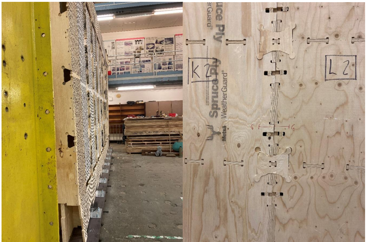
Figure 17 – Failure of the Wall to Foundation Connection (L) and of the Bow Tie Plates (R)
