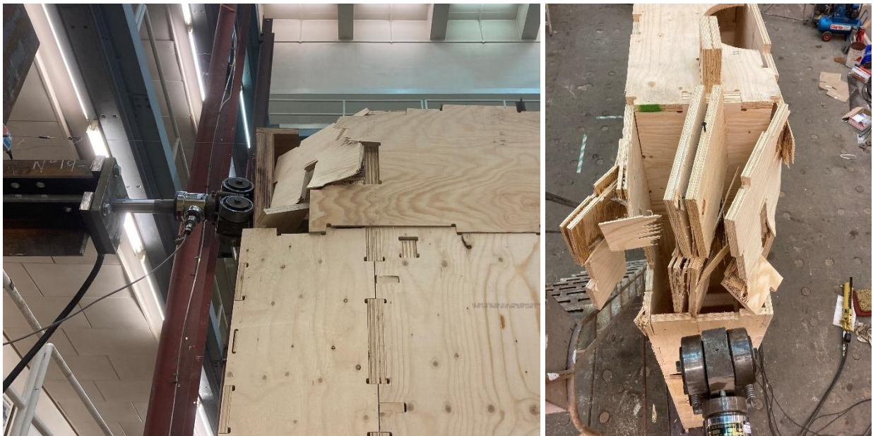
Figure 15 - Localised Compressive Failure of the Wall at the Loading Point on Attempt 1
