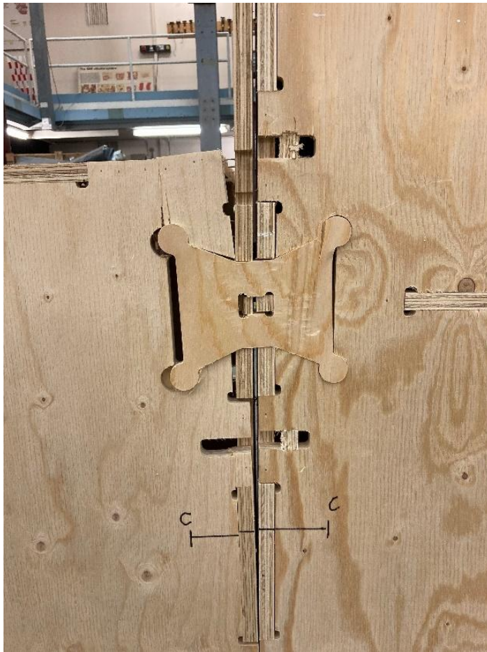
Figure 19 - Failure of the Bow tie plate
