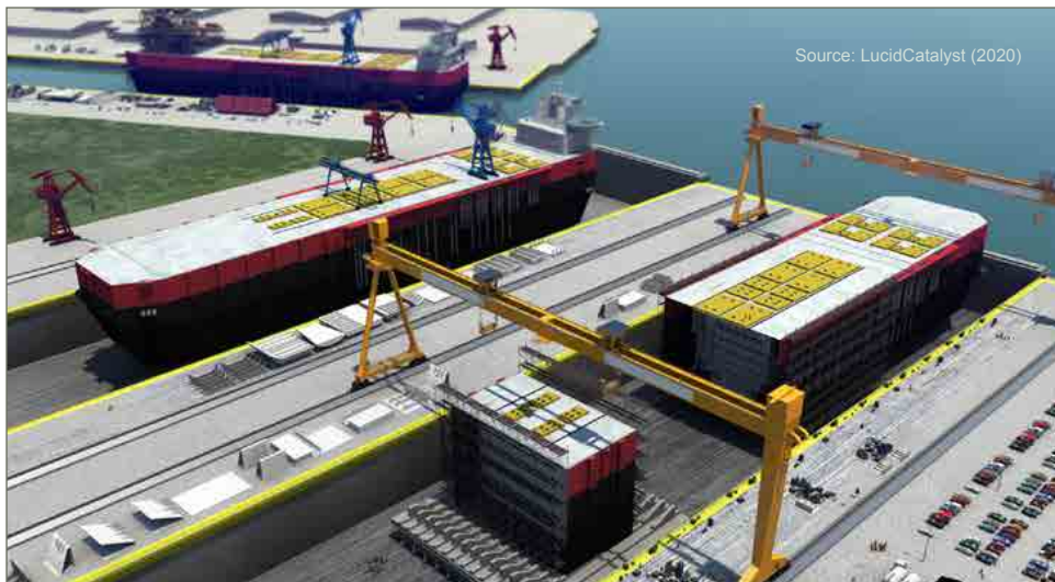
Figure 25. Shipyard manufactured synthetic fuels production facility under construction
