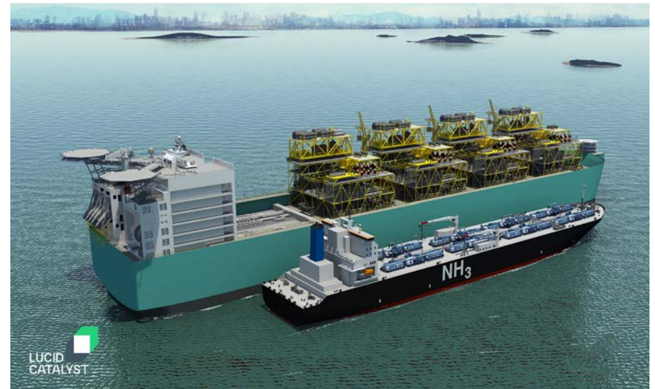
Figure 9. Shipyard manufactured offshore ammonia production platform
