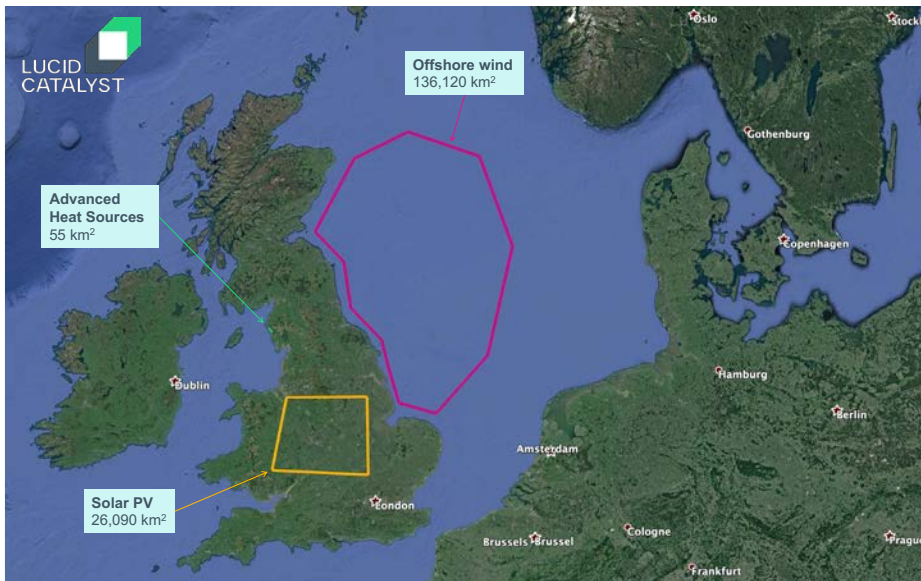
Figure 14. Area that would be required to supply UK's (left) and Japan's (right) current oil consumption with hydrogen from wind, solar, or advanced heat sources
