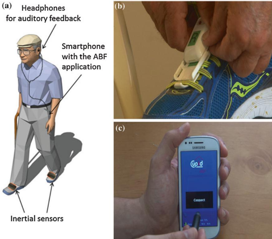
**Fig. 3** a CuPiD system for gait rehabilitation at home composite of three inertial sensing units, a smartphone, and headphones. b Inertial sensors placed on the shoes by means of a dedicated clip. c CuPiD Android application which is able to collect and process the data in real-time and to provide vocal messages to the user
