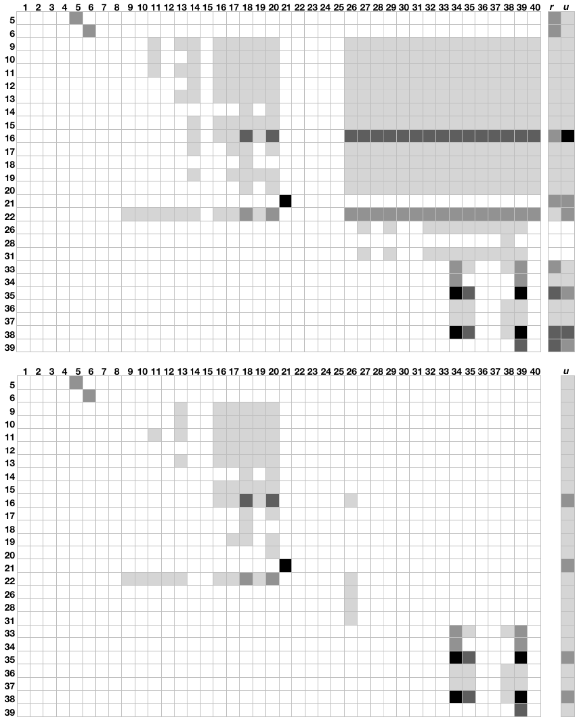
Figure 12: Structural dependency matrix of a M2020 task network of typical size: 40 activities. Up: no task interruptible. Down: all tasks interruptible. Empty rows are not shown. The darker the color of a cell, the bigger the impact.
