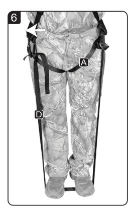
Adjust the SRD Strap so you can step into the loop and then stand up to relieve the pressure on your lower extremities. If the loop is to large for you to stand up, untie the double-overhand knot and adjust the loop size to make it smaller to fit your height.
