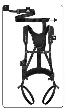
Insert tag end of Tree Strap into the yoke loop of the Full Body Harness tether A. Make sure the flat side of the Slide Adjuster Buckle is facing to the front so the strap can be inserted properly.
