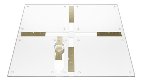
This test device was developed to provide the user with a convenient, quick and accurate way of testing collimation of mammography units. It is very simple to use. Instead of using all those hard-to-find coins, you only use our test tool.
