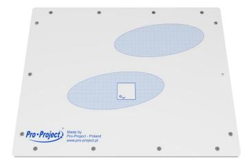
Test grid for testing mammography-cassette film-screen contact.
