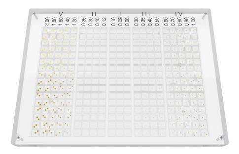
Upgraded contrast details mammography phantom according to European Protocol for quality assurance in Digital Mammography. It can be used to determine if mammographic images indicate objects with very low contrast and very small diameter, to find out the optimum exposure technique, or to compare image quality at various object thicknesses by varying the PMMA thickness.
