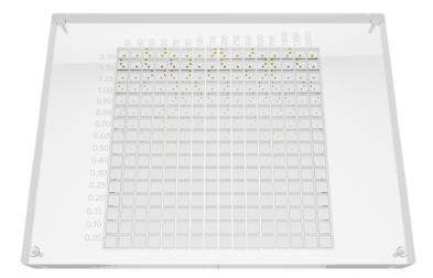
Contrast details mammography phantom according to European Protocol for quality assurance in Digital Mammography. It can be used to determine if mammographic images indicate objects with very low contrast and very small diameter, to find out the optimum exposure technique, or to compare image quality at various object thicknesses by varying the PMMA thickness.
