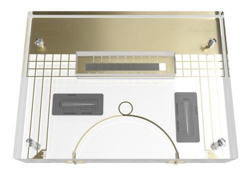
Pro-Euro phantom is used for **monitoring technical parameters** of mammography imaging systems according to the requirements of the "**European Guidelines for Quality Assurance in Mammography Screening**" and IEC 61223-3-2:
