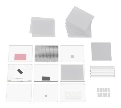
This versatile phantom can be used for monitoring technical parameters of digital mammography imaging systems according to the requirements of the "European Guidelines for Quality Assurance in Mammography Screening" and IEC 61223-3-2:
