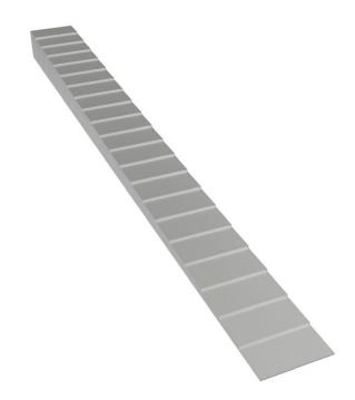
**21 step aluminium wedge** for determination of **the dose reproducibility and sensitometric curve shape, speed and mid-gradient** of mammography X-ray film.
