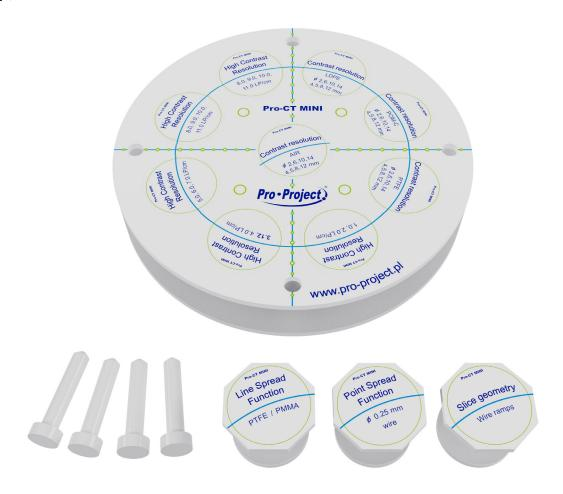
The Pro-CT MINI phantom is a compact CT image quality testing solution. When connected with Pro-CT Dose it may be used for carrying out acceptance and constancy tests of computed tomography systems according to IEC 61223-3-5 and the AAPM (American Association of Physicists in Medicine) guidelines. This phantom consists of a module 16cm in diameter with positioning aids and recesses for test modules.
