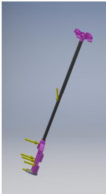
Reaction loads at the claws increased greatly for this case but are not realistic as the drone will not be able to hold its position and forces will be limited.
