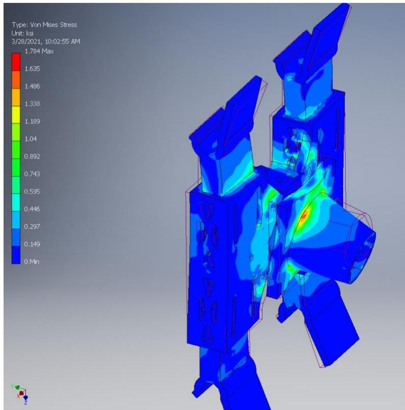
The stress on the frame, claws and pole attachment are modeled conservatively high. The peak maximum stress for this case is 1,800 psi which still provides a safety factor greater than 3.
