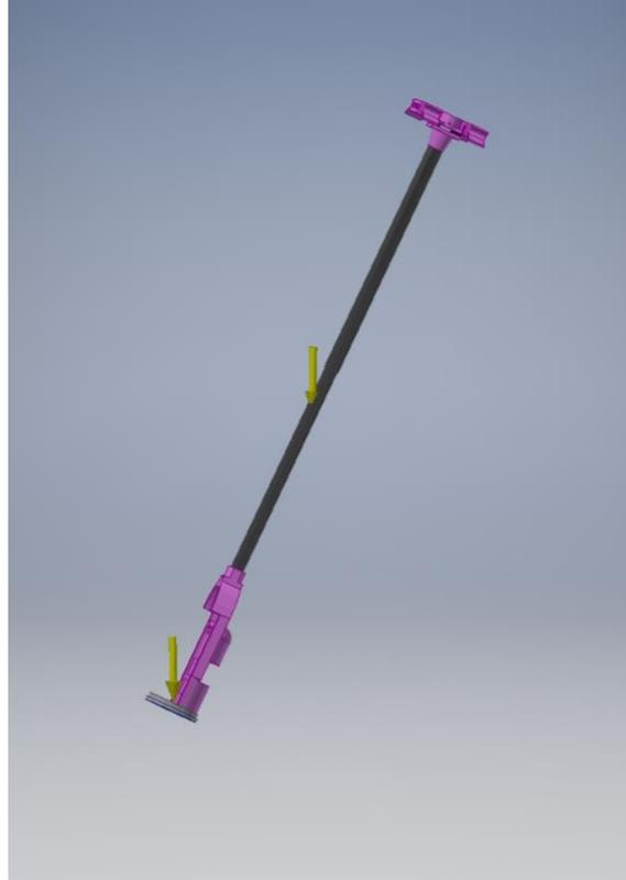
For this case the claws had up and down reaction forces as expected with a magnitude of 2.5 lbs up and .25 lbs down. The inward force against the springs increased to 3.6 lbs at the higher loaded end and .9 lbs at the other end. Axial forces were unbalanced with 1.0 lbs on the loaded end and .6 lbs on the other.
