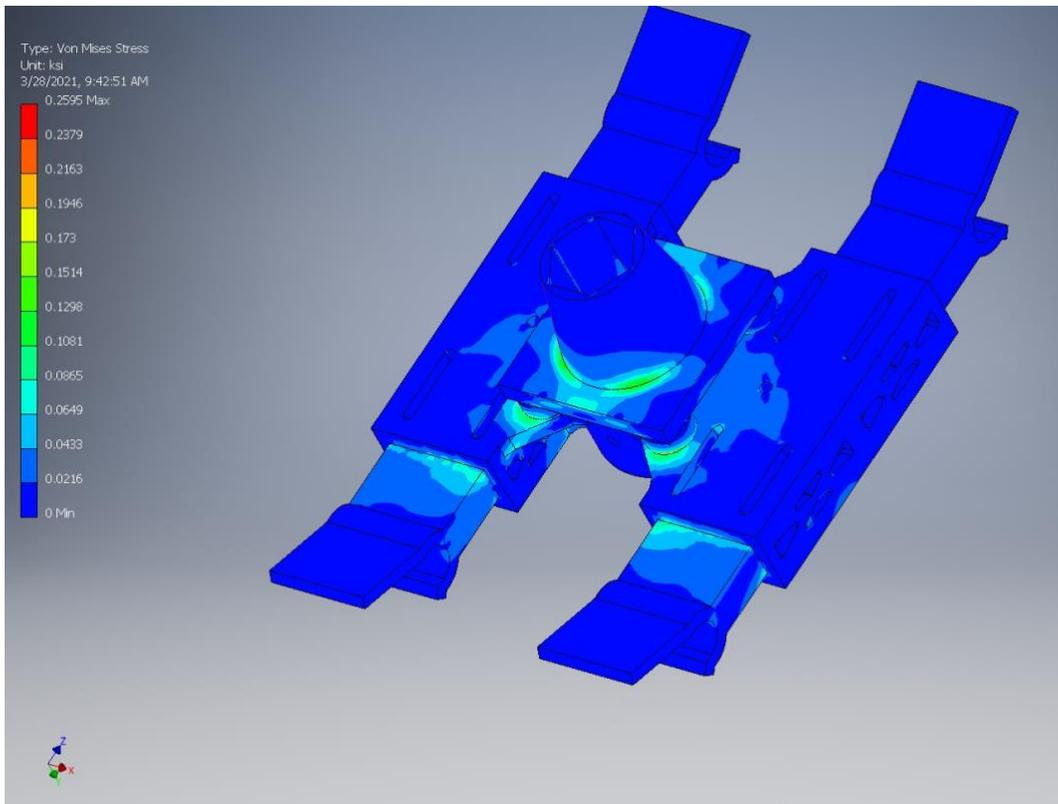
The frame, claws and pole attachment peak stresses are all under 300 psi which provides a safety factor of 20.
