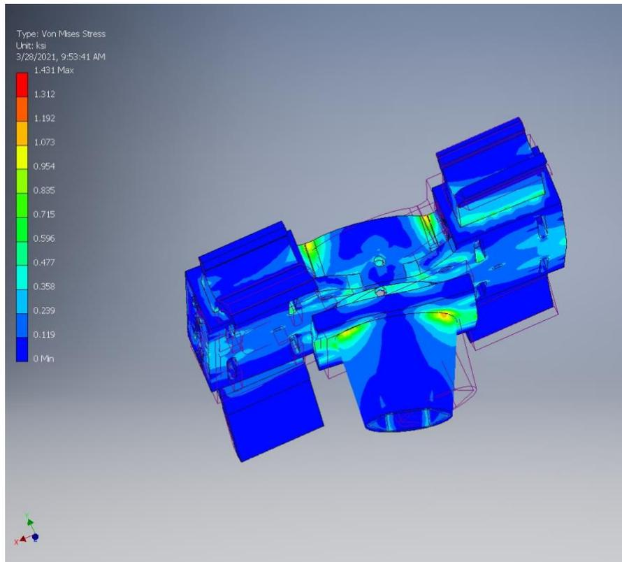
The stress on the frame, claws and pole attachment are modeled conservatively high. The peak maximum stress for this case is 1,400 psi which still provides a safety factor of 4.
