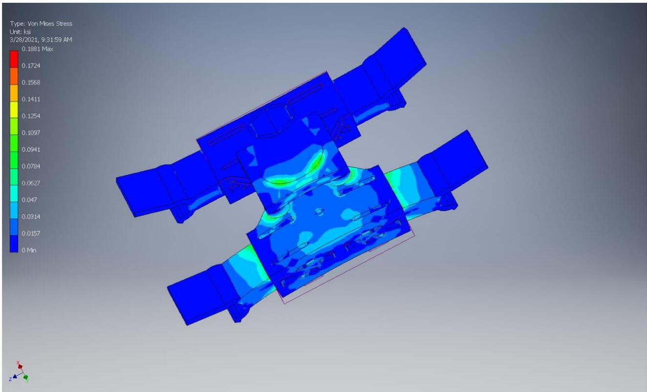
The stresses on the frame, claws and pole attachment are peak of 188 psi providing a safety factor greater than 30.
