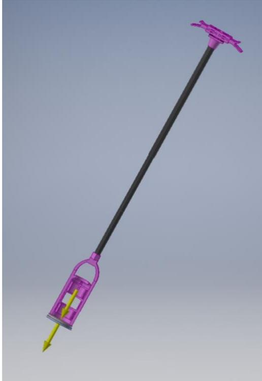
The total reaction load in the Y direction for this case was 4 lbs. Claw inward reaction forces (compressing the spring) are 1.5 lbs each claw equal and opposite across the Top Frame. Each claw also has axial reaction forces of 1.3 lbs in opposing directions.
