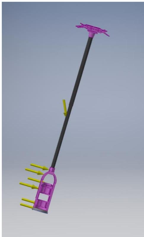
Reaction loads at the claws increased greatly for this case but are not realistic as the drone will not be able to hold its position and forces will be limited.
