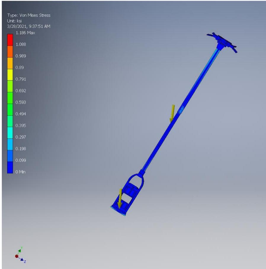
The reaction forces for this case are 2.3 lbs up on one side and 1.1 lbs down in the vertical direction. The inward forces are 1.6 lbs inward and 1.1 lbs outward. Axial forces are 1.6 and .1 lbs.
