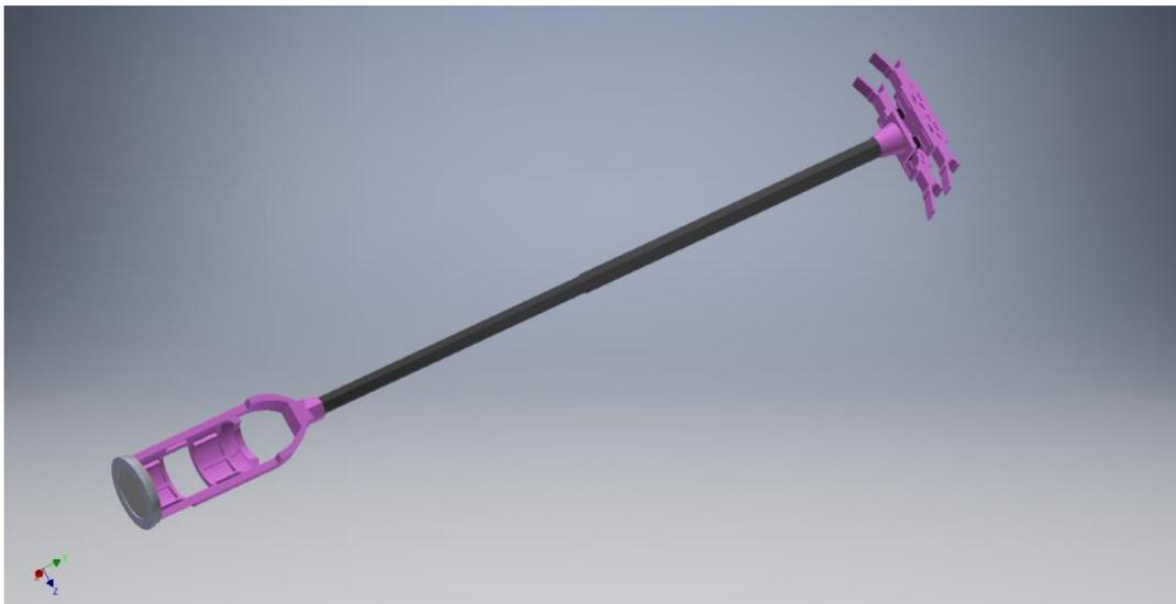
The stripped down water basket assembly is shown below. The bottle cage door was removed as it didn't seem to add structure using slip pin hinges and button closures, the weight of the door and the bottle (also not modeled) was added in with the water load weight.
